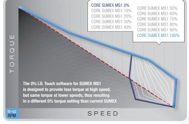
FIGURE 2: New SUMEX MS1 Torque Profile (5400-130-000S1)
