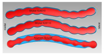
**Figure 4:** Implant patch (marked red) which is considered for the fitting analysis
